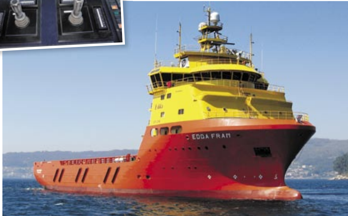
Norwegian supply vessel Edda Fram was the first ship to put to sea with the new Voith roll stabilization system. The inset above left shows the Bosch Rexroth controls on the bridge.
